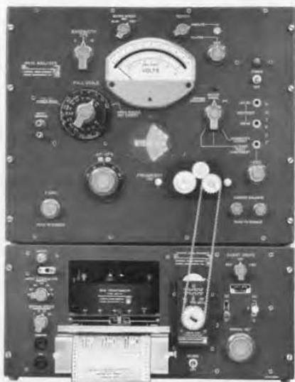
Figure 4. View of the Type 1910-A Recording Wave Analyzer, consisting of the Type 1900-A Wave Analyzer and the Type 1521 Graphic Level Recorder.
